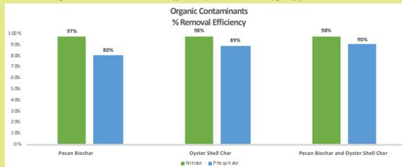
Figure 5. Organic contaminants removal efficiency based on the type of filter media used
