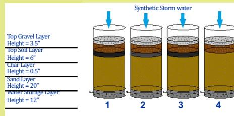
Figure 2. Bioretention columns used to test effectiveness of filtration materials. (1) Pecan Biochar (2) Oyster Shell Char (3) Pecan Biochar and Oyster Shell Char (4) Sand only
