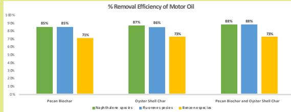
Figure 4. Motor oil removal efficiency based on the type of filter media used
