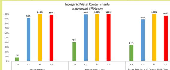
Figure 6. Metal contaminants removal efficiency based on the type of filter media used
