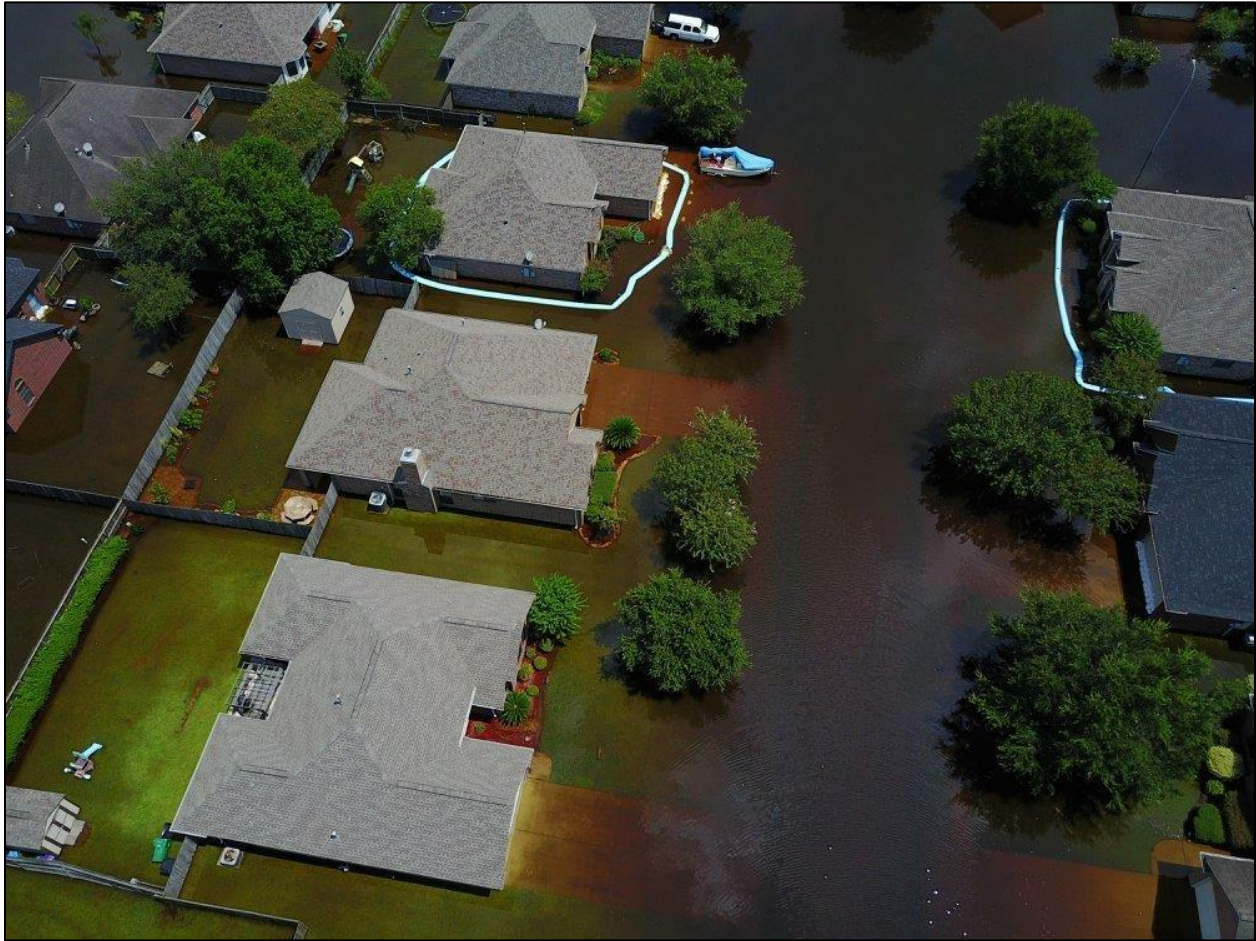
Figure 19b. Clear water is evident in the flooding of the streets and lawns in Richwood. The clarity of the water is indicated in the ability to see the driveway surfaces and the lawn grass. The clarity of the water draws into question the claim by Grounds (2019) that the flooding of Richwood resulted from the overflow of the Brazos River (compare with muddy water of Brazos River in Fig. 18). Still shot of drone video taken between August 30 and September 1, 2017, and provided by Matías J. Adrogué, PLLC.
