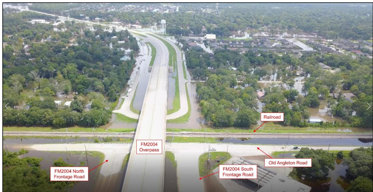
Figure 9. The flood water mostly did not flow directly over the highway FM2004 or the railroad. View looking to the east (compare with veer of FM2004 to the left (northeast) in Fig. 3). It is most likely that the flood water crossed the railroad under the bridge over Bastrop Bayou and crossed FM2004 through culverts that connect the “East Ditch” and “West Ditch” on the north and sides of the highway (see Figs. 3, 10-11). Figure modified from still shot at 4:14 of drone video labeled Before-8 taken on or before September 3, 2017, and provided by Matías J. Adrogué, PLLC.
